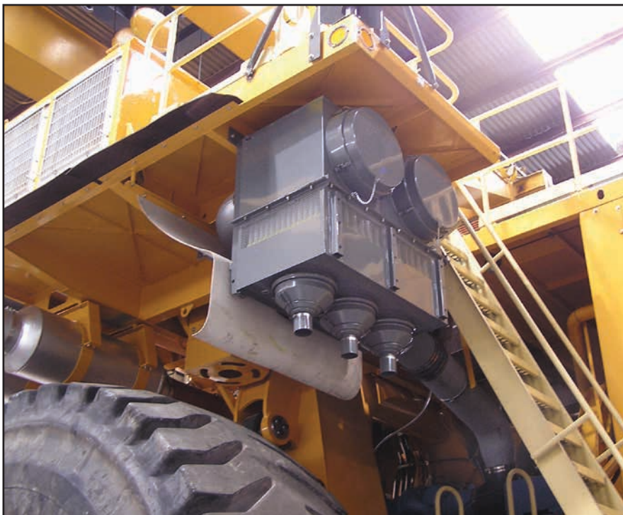
The large, massive mining vehicle in the picture above is an ideal match for the Donaldson SSG Air Cleaner.
