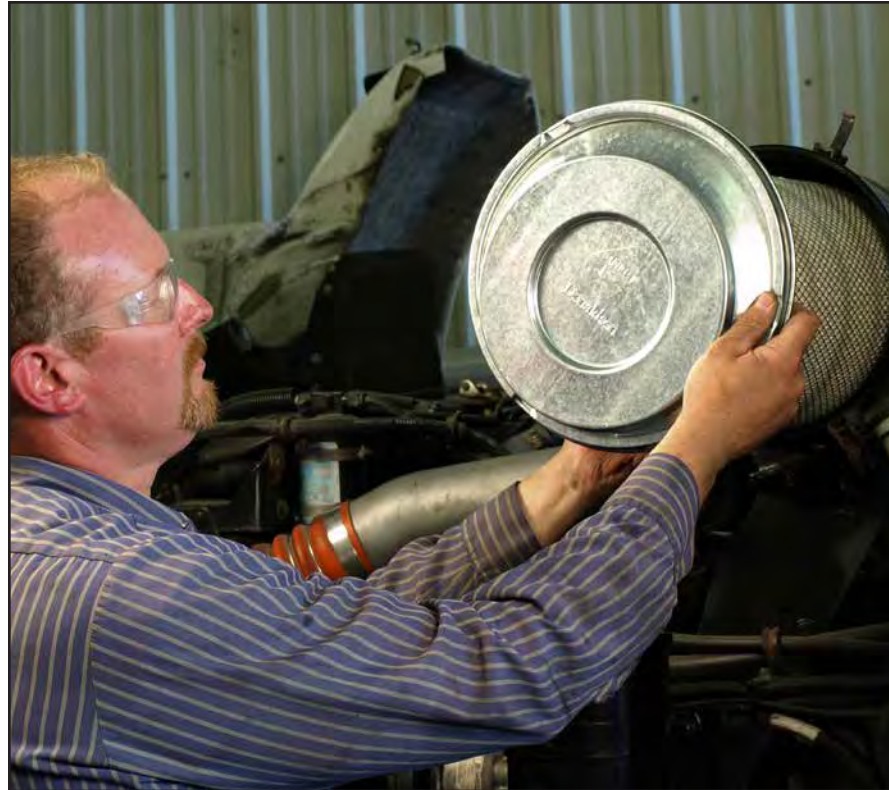
The latched service cover on the ECG Konepac allows for easy access to the filter for change out.
