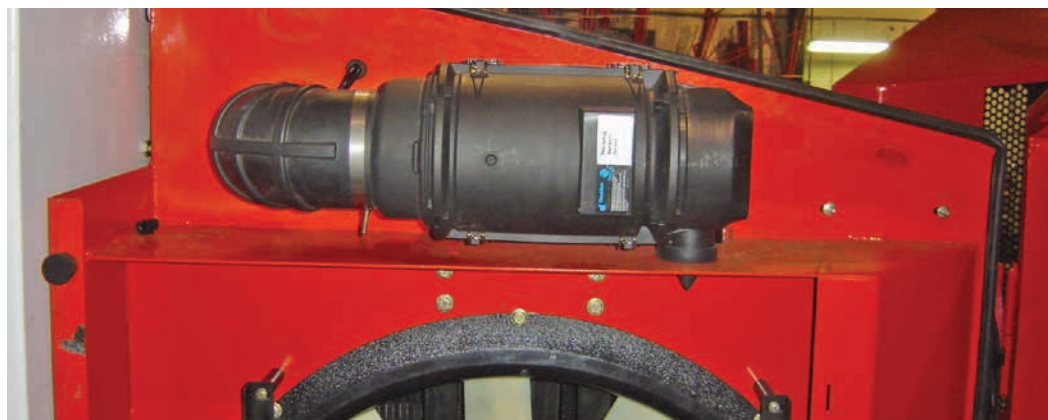
A PSD10 mounted horizontally was the equipment manufacturer's choice on this diesel-powered (285 HP @ 2,000 RPM) feller buncher.
