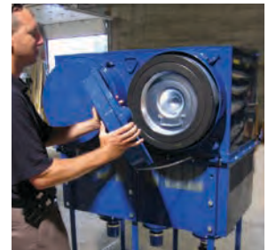
No more bolt to unscrew for a filter change — simply unlatch the cover and let it hang from the housing during service.
