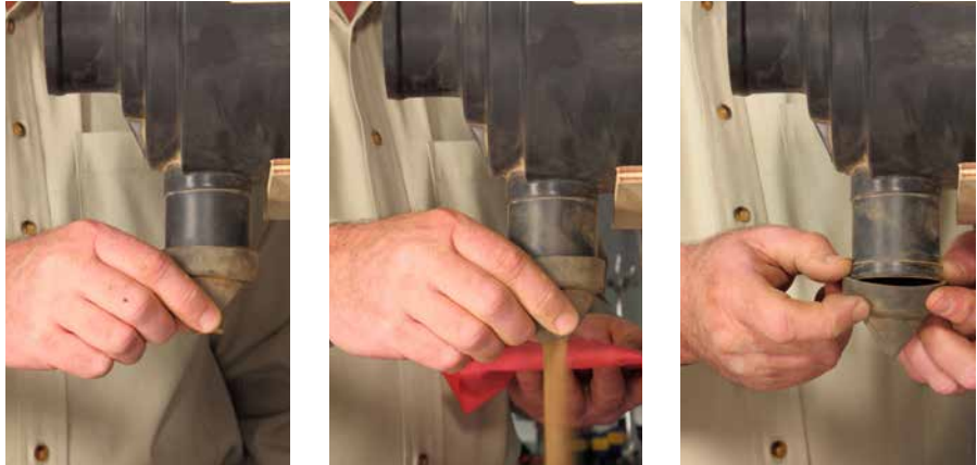
If your air cleaner is equipped with a Donaldson Vacuator™ Valve, make sure your routine filter service includes checking it to make sure it's in good condition and not plugged. If the Vacuator Valve is plugged, clean it.
