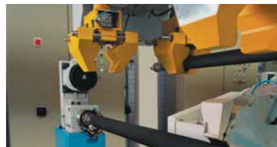
Because even a 1mm variation in wall thickness can impact hose life by 25%, every hose is precision machined to ensure repeatable performance.
