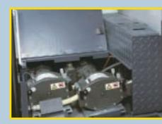
Installed on the UV varnish tower coater of MAN Roland R700 series printing presses, twin baseplate-mounted 701 pumps have reduced downtime and increased production speed. One pump accurately metres the water-based varnish from a container to a weir on the press, the other scavenges excess varnish for re-circulation.
