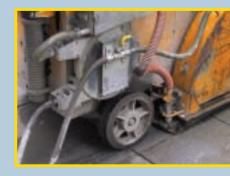
Watson-Marlow Bredel peristaltic pumps are used wherever quality and reliability are paramount – as here, powering coolant flow in a concrete-cutting machine in Japan. The pump is the circular housing, centre.
