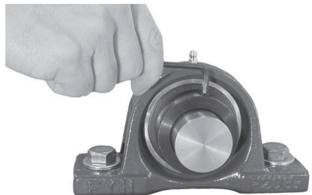
Fig. 14.10 Installing eccentric locking collar
